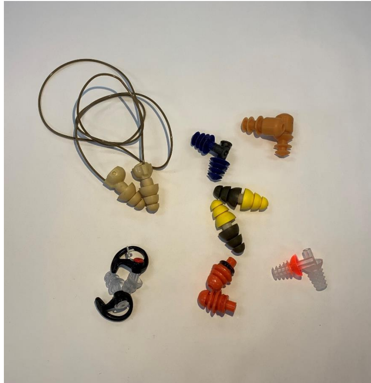
Figure 5.7 - Level-dependant ear plugs Constant sound can be transmitted down the tube to the ear but sharp rise time impulse noise is attenuated by an insert
