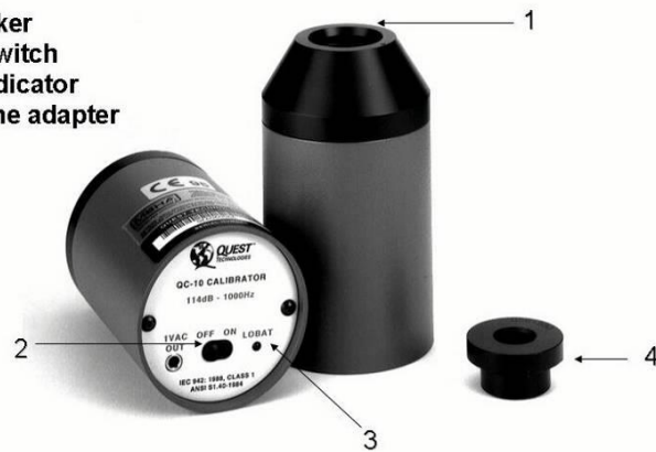
Figure 3.6 – Typical acoustical calibrator used for field calibration
