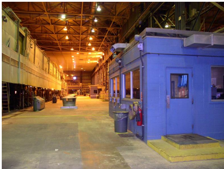
Figure 4.6 - Acoustical control room and noise refuge in a paper manufacturing facility
