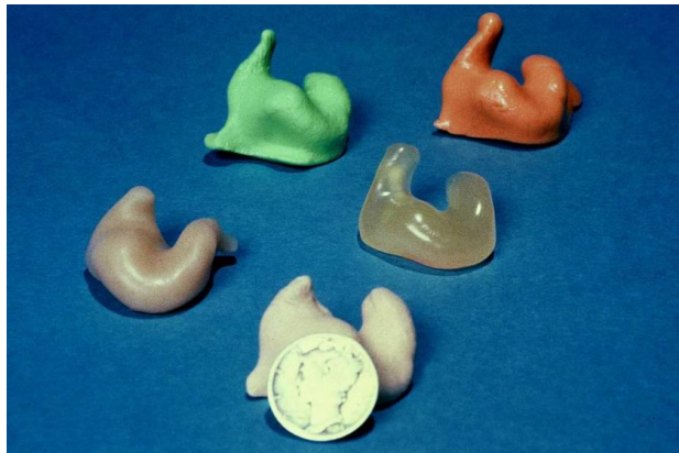
Figure 5.4 – Five Custom-molded Plugs made for the same ear canal by five different technicians
